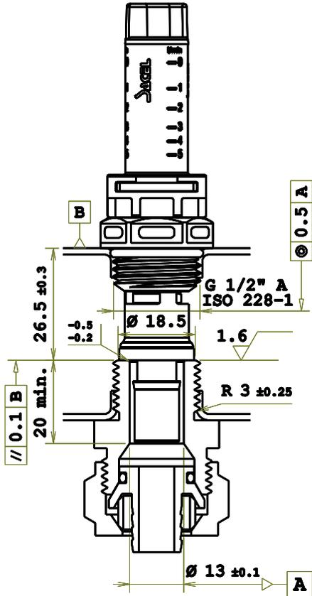
The manifold with the installed flow meter must always be positioned on the supply side, while the shut-off valve must be mounted on the return line of the connected hydraulic system. An incorrect placement of the manifold can cause system anomalies, preventing the proper functioning of the flow meters, which must operate exclusively in suction mode.
