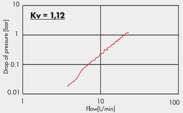
The kVS value is influenced by the type of counterpart used and the geometric configuration of the distributor. For this purpose, you will receive a drawing from us with the necessary connection dimensions.
